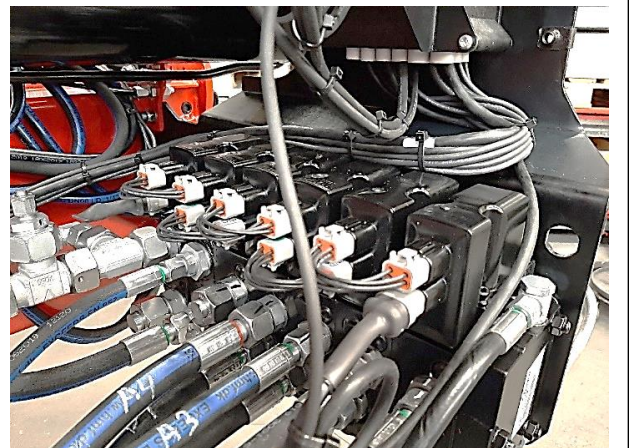
PVED CC, CANopen electric activations with corresponding loop cables and termination.
